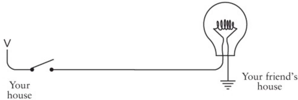
The V stands for *voltage*, but it could also stand for *vacuum*. Think of the V as an electron vacuum and think of the ground as an ocean of electrons. The electron vacuum pulls the electrons from the earth through the circuit, doing work along the way (such as lighting a lightbulb).
