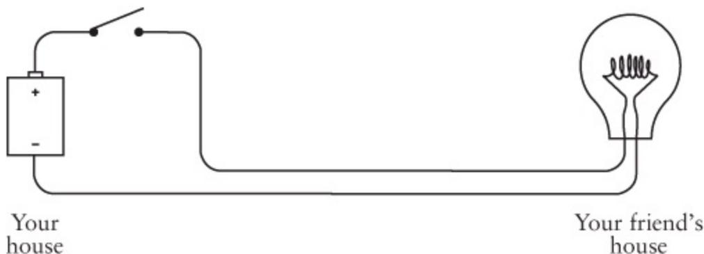
Although I'm showing only one battery, you might actually be using two. In this and future diagrams, this will be an off (or open) switch:
